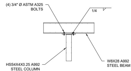
7 COLUMN TO BEAM CONNECTIONS - TYPICAL
