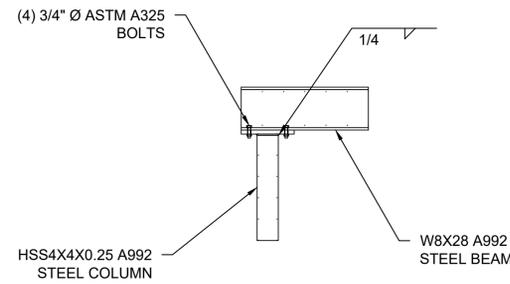
6 COLUMN TO BEAM CONNECTIONS - TYPICAL
