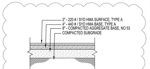
5 ASPHALT PAVEMENT DETAIL
