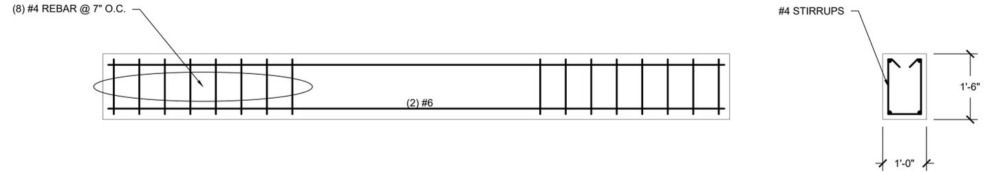
4 CONCRETE BEAM DETAIL - BEAM CB1
