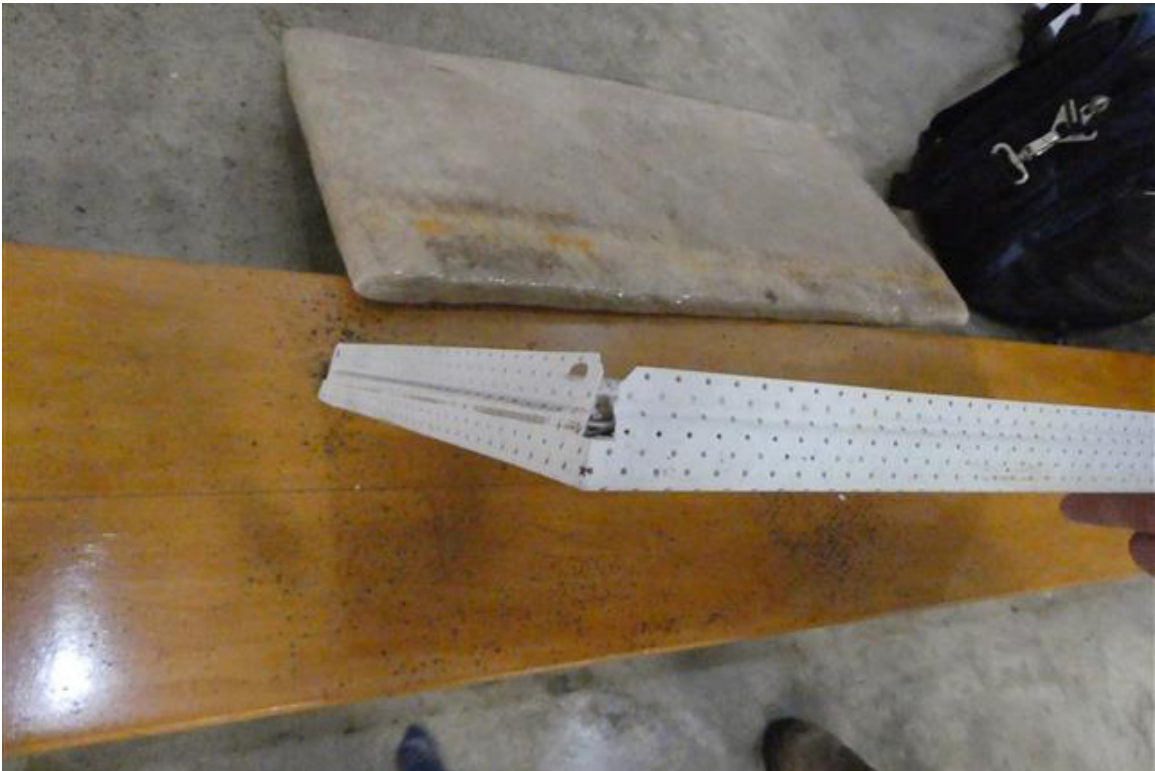
Photo 10 - Both the ends of the tile and the spline are grooved. The tiles nest to each other and the spline, holding them in position.
