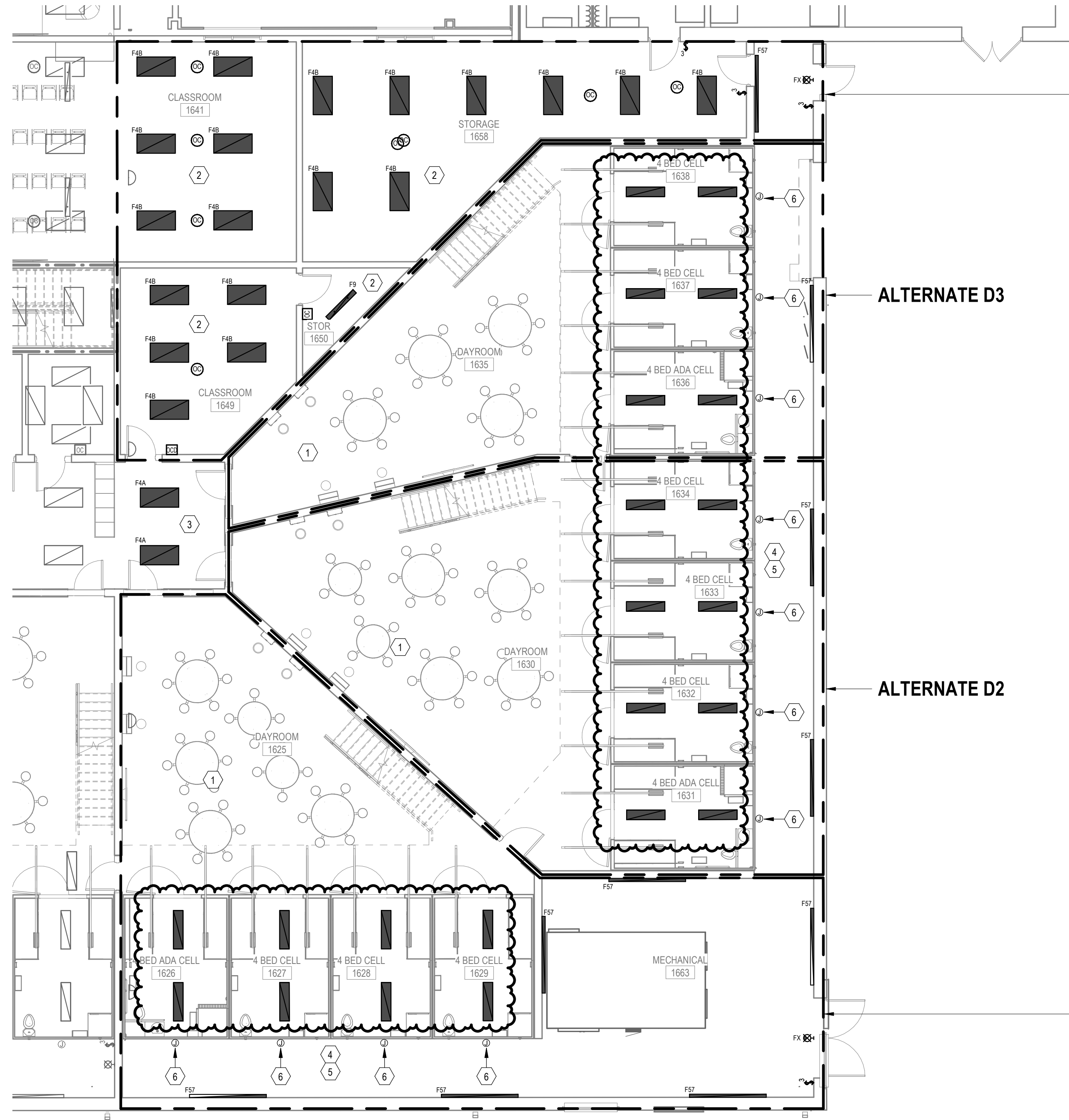
2 FIRST FLOOR LIGHTING PLAN - UNIT D, ALTERNATES D1-D3 1/8" = 1'-0"
